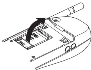
⑤ Slide the card carefully into the holder. Ensure that the bevelled corner is up-
